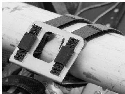
1: FACEPLATE OF THE BRACKET ON A WING RIGGER WITH PADS FOR SMARTPHONE
